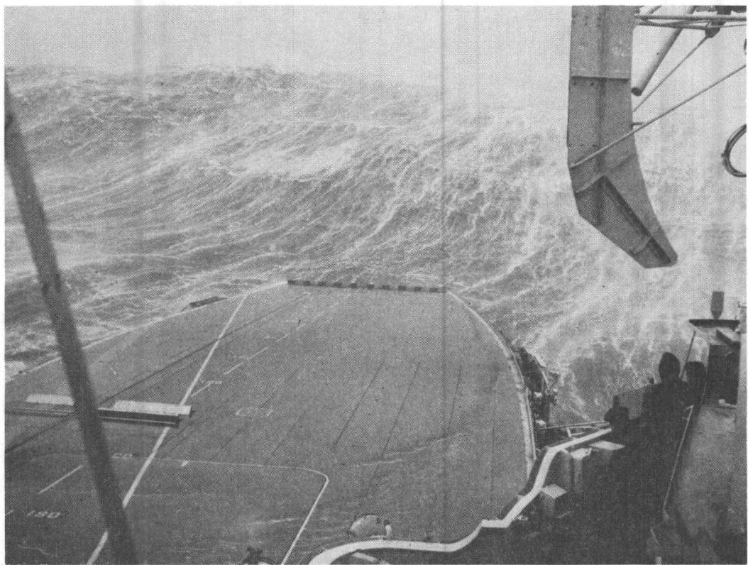
HMCS *Bonaventure*, a Canadian aircraft carrier, in heavy sea northeast of the Azores on 6 December 1959. During the height of the storm, winds were 34 m/s (68 knots) with gusts up to 45 m/s (90 knots) and waves reached heights of over 15 m with some exceeding 18 m. Compliments of the Department of Defence, Ottawa.
