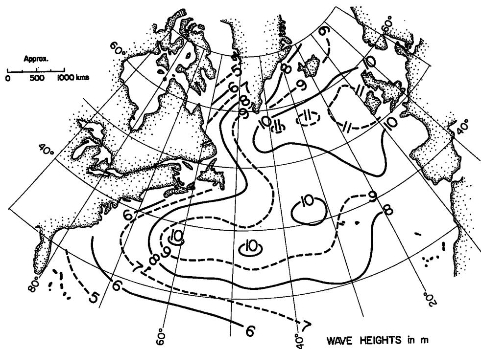
Figure 20. One-year (1970) Largest Observed (Significant) Wave Heights
