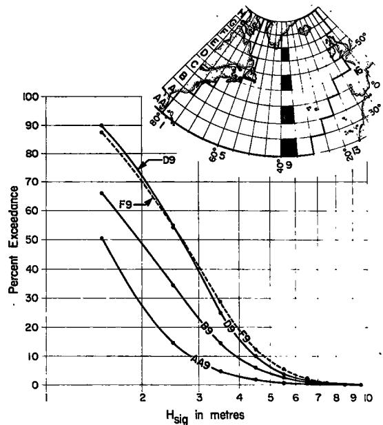
Figure 19b. Wave Height Exceedance Diagrams from South to North
