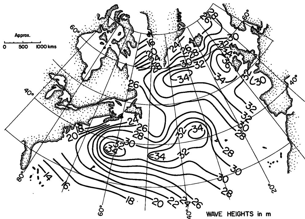
Figure 25. 100-year Maximum Wave Heights (Design Waves )
