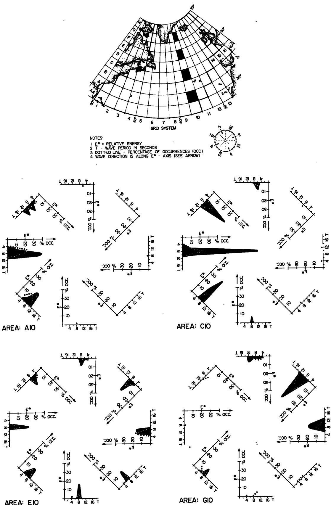
Figure 15. Directional Energy Spectra from South to North Along mid-Atlantic in January
