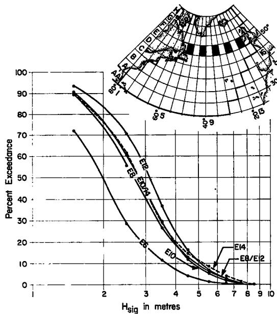
Figure 19a. Wave Height Exceedance Diagrams from West to East
