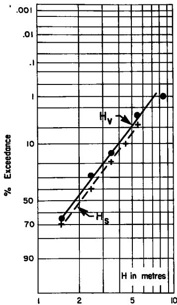
Figure 10. Visual Observations versus Recorded Measurements
