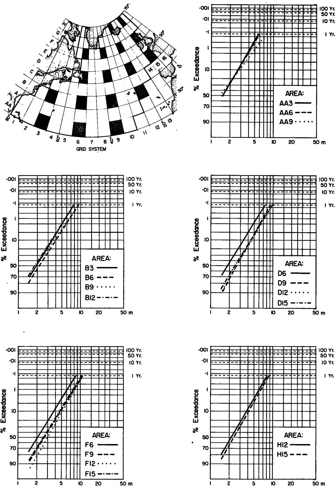
Figure 18. Samples of Wave Height Exceedance Diagrams Across the Atlantic
